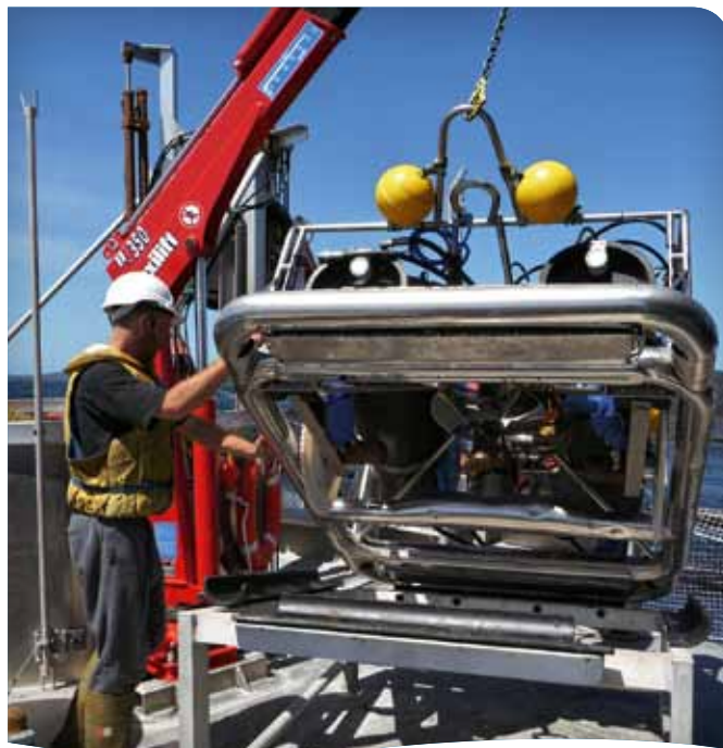
MIC netcleaner being placed in cradle after being removed from cage
